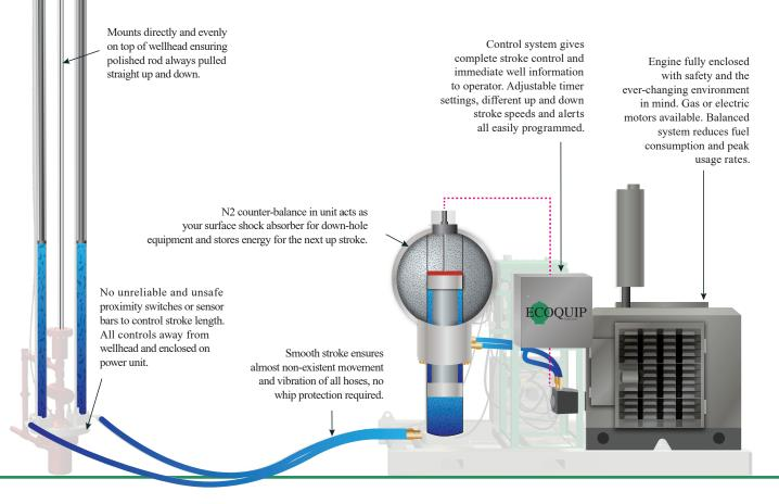
Ecoquip 9000-6X model hydraulic pump jack 🌒 158" stroke length/ 7-8 SPM / 35,000lbs max load 🌒 Patented design from Calgary, Alberta
